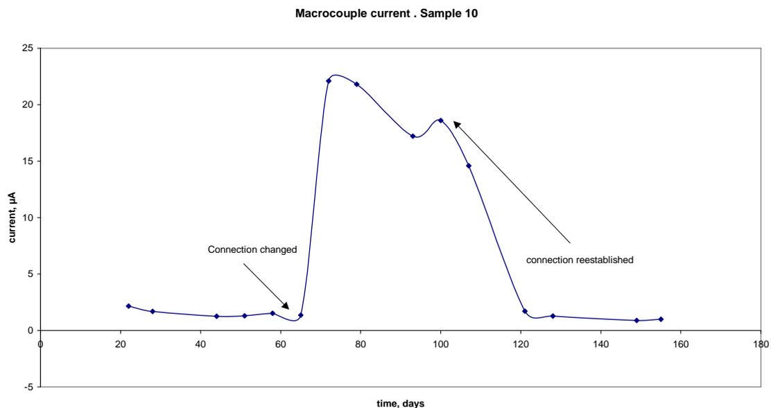
**Figure 7:** Influence of cathode material on the macrocouple current
