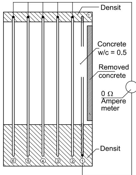
**Figure 1** Experimental model. See also Figure 3 and Figure 4.
