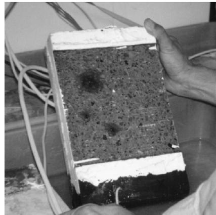
**Figure 4** Experimental set-up for group 3 and group 4. The dark areas are red corrosion products.
